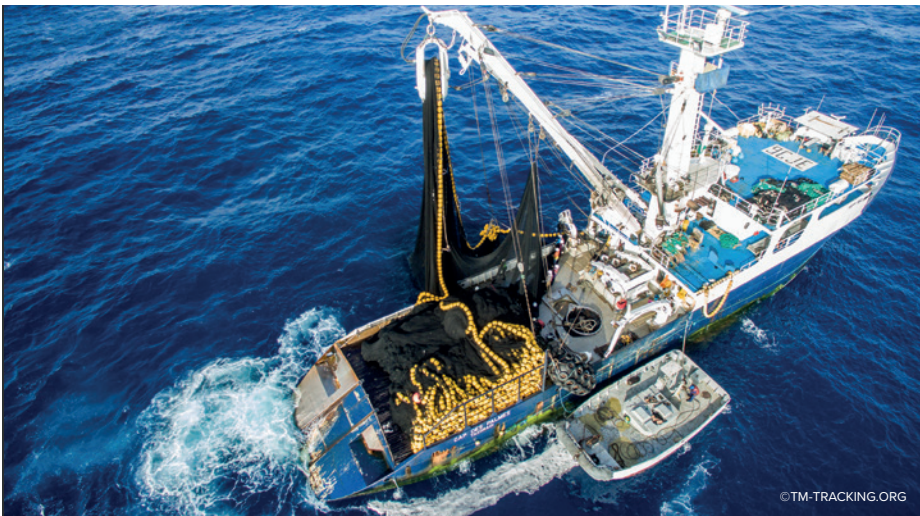
A purse seiner in the process of hauling the net after it has been 'pursed' around a school of tuna.
