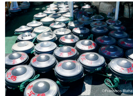
FAD transponders. Each will be attached to a FAD and transmit information about the fish that are present under the FAD, as well as positional location.
