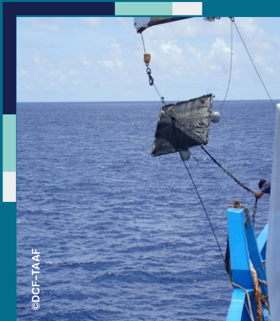
Figure 8: A drifting FAD in the process of being deployed by a purse seine vessel. Visible is the square surface raft and floats, to which a tracking buoy will be attached, as well as the 30–80 m subsurface cord.
