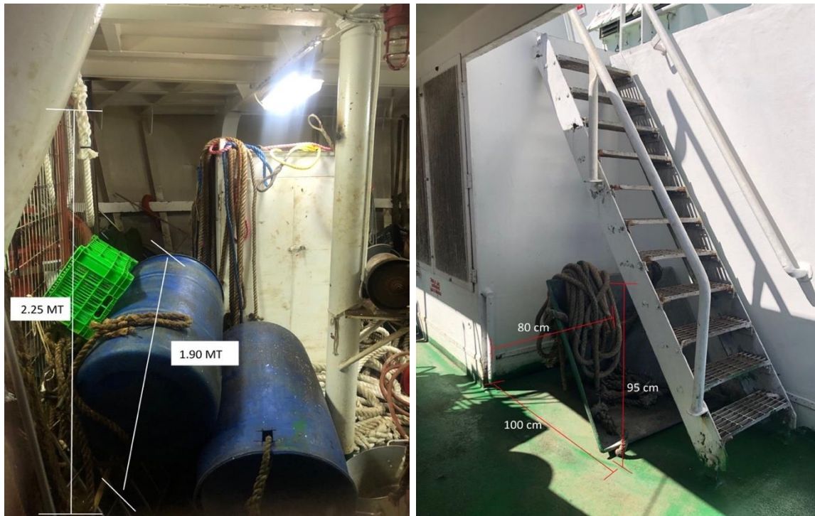
Figure 15. Detail and dimensions of recommended sites for installation and anchoring of seabird stations on the deck of purse seine vessels targeting jack mackerel, south-central Chile.
