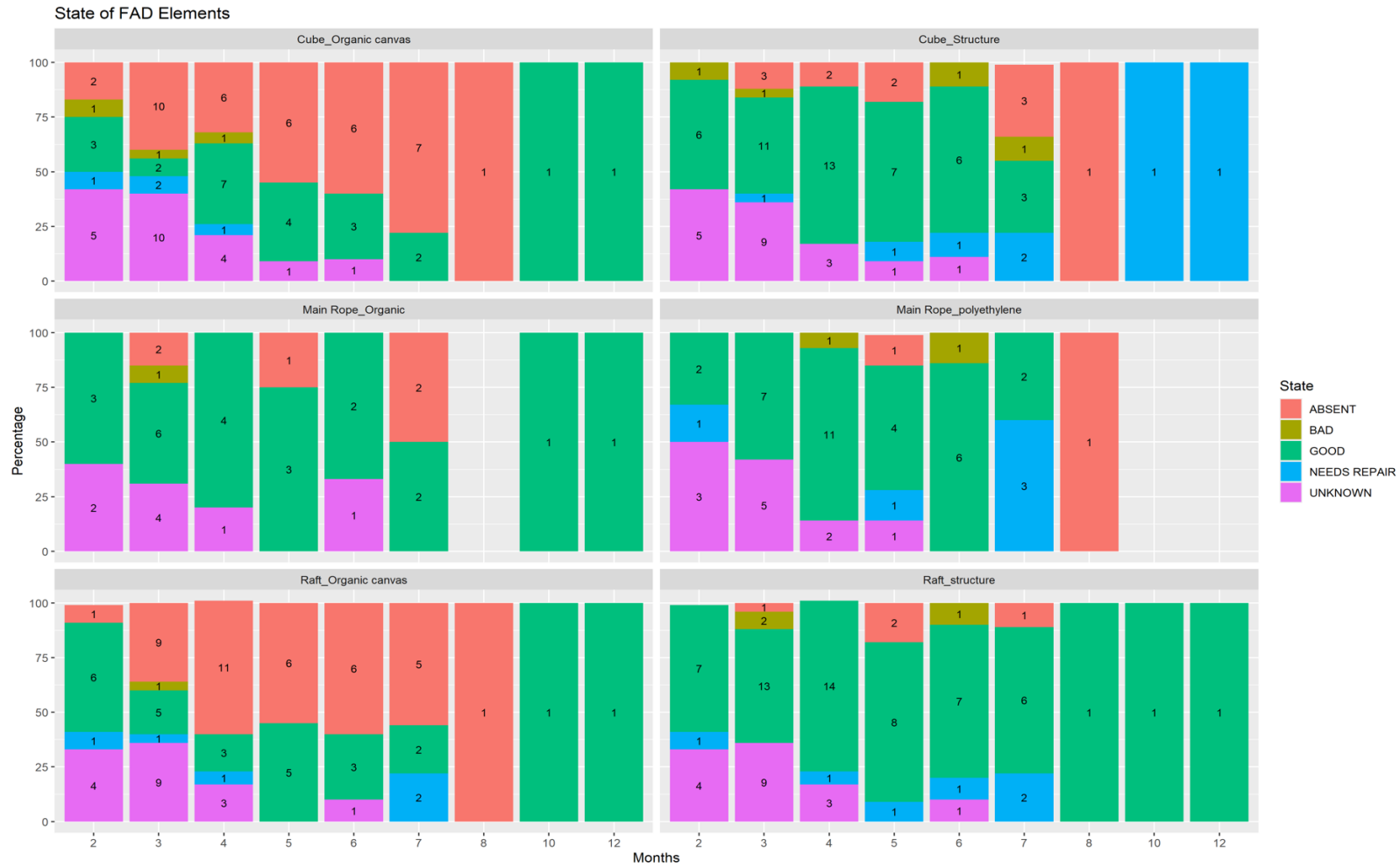
Figure 8. Degradation of the different components over time in months (X-axis). State 1 = good condition (green), State 2 = needs repair (blue), State 3 = bad (yellow), State 4 = component not present (red) State 5 = unknown (purple). Number of observations are written in the columns.
